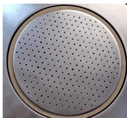
Fig. 1. The photo of the shower nozzle (top) electrode
