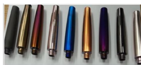
Fig. 3. Photography of coloured Ti/Ti-O layers deposited on polymer substrates by used a PMS and GIMS method
