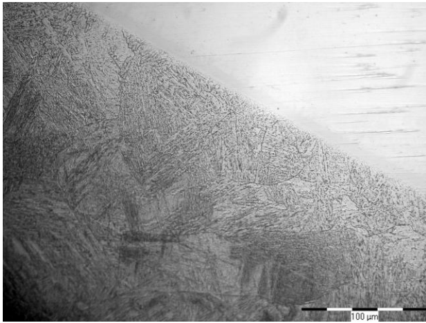
Fig. 4. HAZ structure ( \times 400 ) in the vicinity of the fusion zone when surfacing with TIG by a fixed arc
