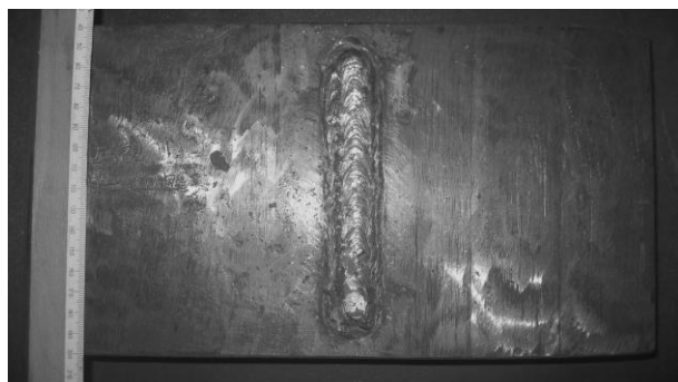
Fig. 13. Simulative repair welded joint of steel 15Kh2MFA
