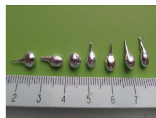
Fig. 3. The samples of zinc granules after pouring
