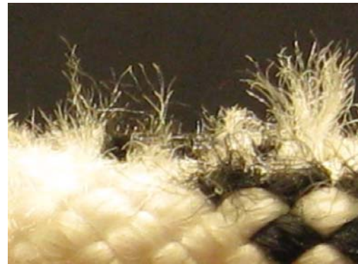
Fig. 5. Enlarged photos of the rope sample: a) thin TiO_x film covered, b) unmodified
