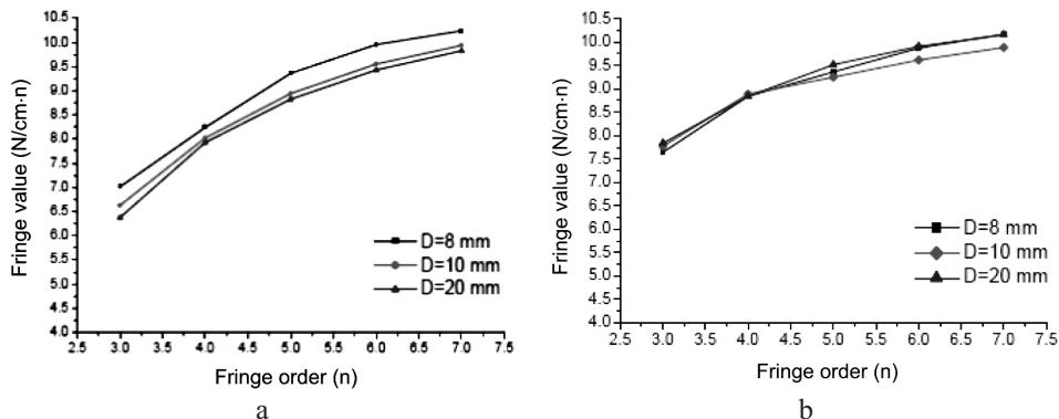
Fig. 5. Experimental fringe value vs. fringe order dependences for PCM disks of 8, 10 and 20 mm in diameter before (a) and after (b) annealing.
