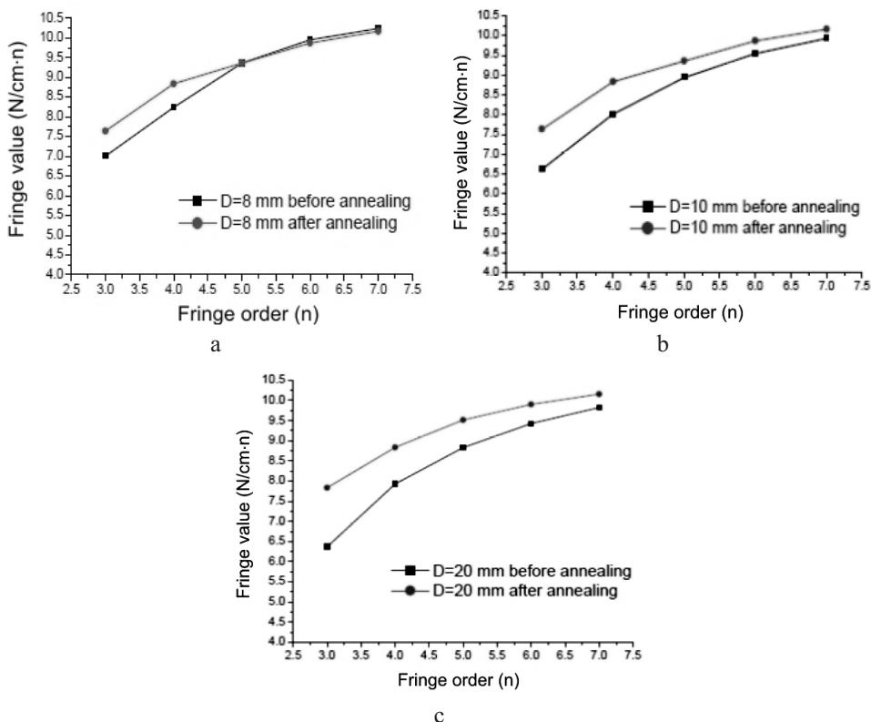
Fig. 6. Experimental fringe value vs. fringe order dependences before and after annealing for PCM disks of 8 (a), 10 (b) and 20 mm (c) in diameter.
