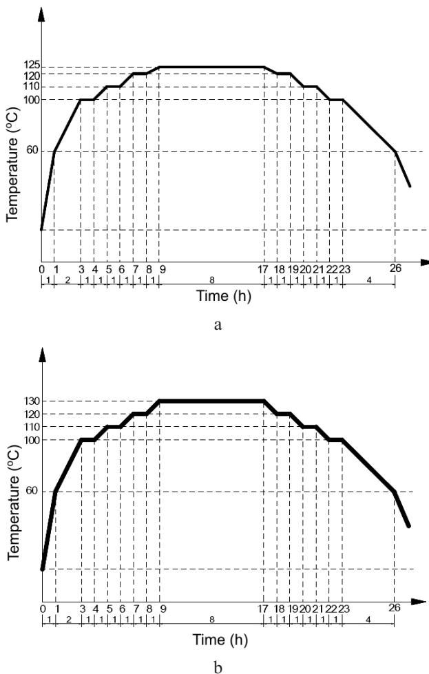
Fig. 2. Annealing curves for disks of different diameters: 1 to 3 mm (a) and 4 to 8 mm (b).
