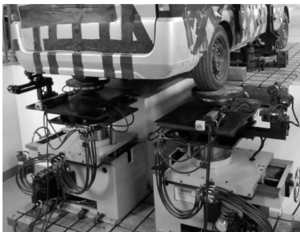
Fig. 10. Static calibration test system.
