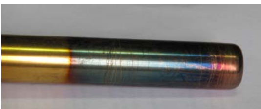
Fig.5 Cathode photo after performance. Diameter of cathode rod 20 mm
