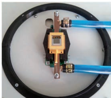
Fig. 2. Measuring system in general and an example of how a 640x512 EMCCD chip is connected to the system
