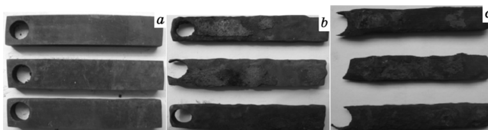
Fig. 2. The macromorphology of corrosion products of L360QCS formed at different temperatures: 30°C (a), 50°C (b), 90°C (c).
