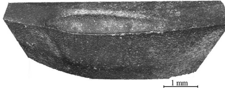
Fig. 6. 3D view of worn BCBN tool.
