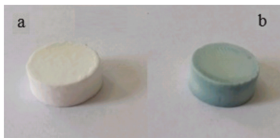
Fig. 3. The view of \text{Ca}_{10}(\text{PO}_4)_6\text{F}_2 ( T = 1250^\circ\text{C} , \tau = 9 h) samples before (a) and after (b) electron irradiation process.
