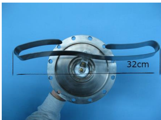
Fig. 1. T-shaped antenna mounted on 160 mm flange
