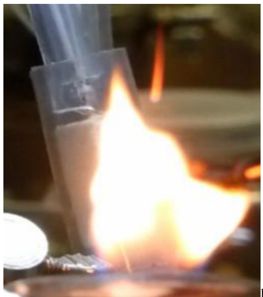
Fig. 7. Photo of paraffin combustion: corona discharge – “off” (a); corona discharge – “on” (b)
