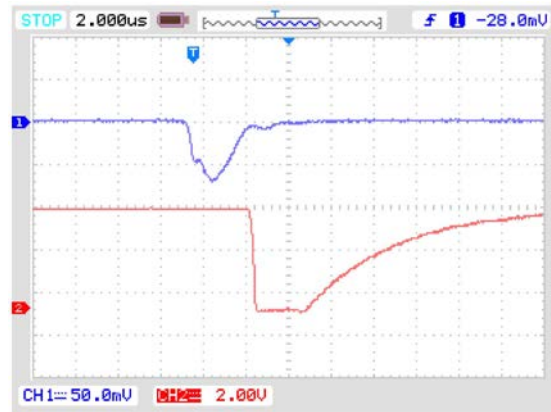
Fig. 4. Oscillogram of signal transmitter and light pulse receiver Beam 1 – the current passing through the light diode; Beam 2 – output pulse after the converting receiver of light pulses
