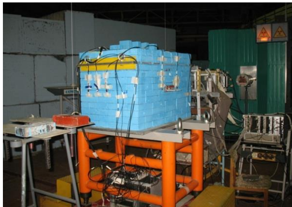
TA Quinta at the irradiation position in the F3 focus of the Nuclotron accelerator
