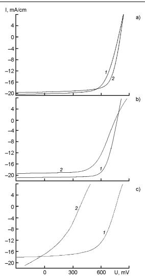
Fig. 2. Light CVC of SC on CdTe base:
