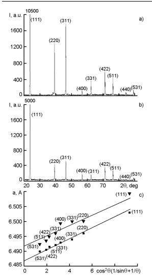
Fig. 1. Structural researches of CdTe base layers in structure the polyimide film/ITO/CdS/CdTe/Cu/Au CS: (a) XRD pattern of CdTe layer in SC structure deposited on unannealed ITO layer; (b) XRD pattern of CdTe layer in SC structure deposited on annealed ITO layer; (c) Lattice period of CdTe layers: ■ — CdTe layers in SC structure deposited on annealed ITO layer; the same on unannealed ITO layer.
