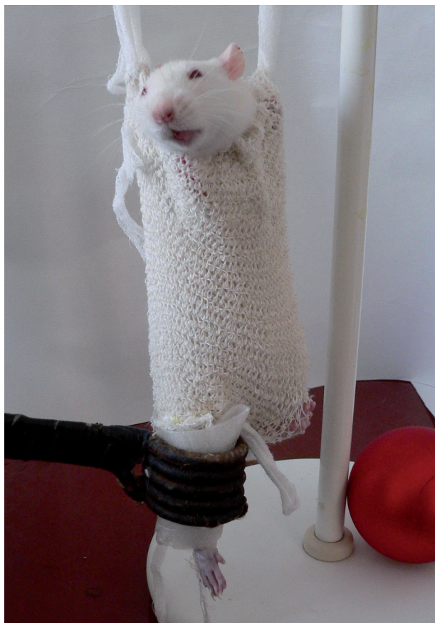
Fig. 1. Photograph of rat in the special created net-hammock (the femur is located in the coil of magnetic field generator)
