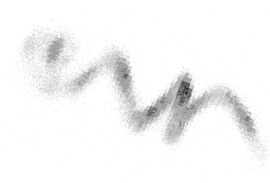
Fig. 6. A 3D image of a variable pitch helix. The diameter of the tube bent into helix is 1 mm.
