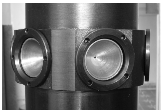
Fig. 5. The main assembly of multi-pin-hole collimator.
