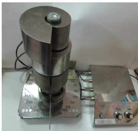
Fig. 2. Device for determining the point GRS direction with an asymmetric absorber, an absorber shaped as a coaxial cylinder, a sector absorber, and an analyser of gamma-radiation impulses.
