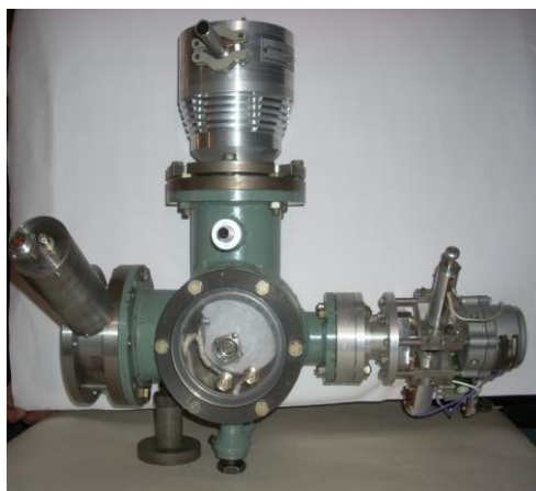
Fig. 1. Chamber for the study of the properties of construction materials
