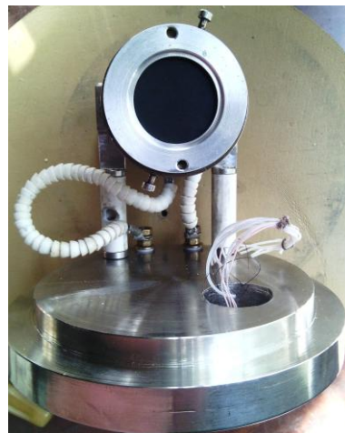
Fig. 7. A cell for measuring the electrophysical properties of materials under a beam He^+ with attached sample
