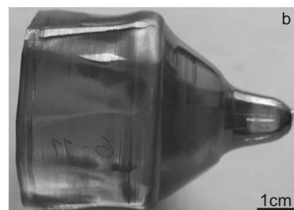
Fig. 3. BGO crystals grown using: a — setup Fig. 1b, b — setup Fig. 1c.
