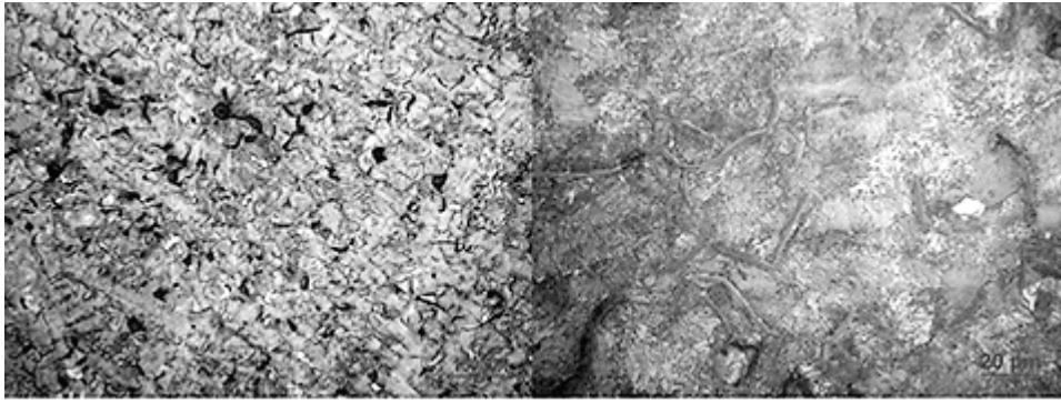
Fig. 4. Structure of the ventilated brake disc from cast iron (etched—Nital 3%).
