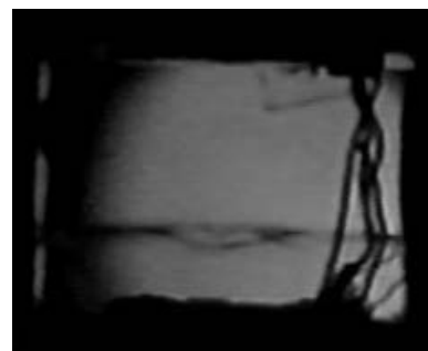
Fig. 1. Melting of ^4\text{He} crystal induced by sound wave from the liquid side.
