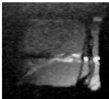
Fig. 3. Melting of ^4\text{He} crystal induced by sound wave from left to right.
