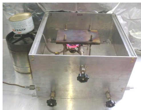
Fig. 5. Working hydrogen generator HG-1 with hot screen
