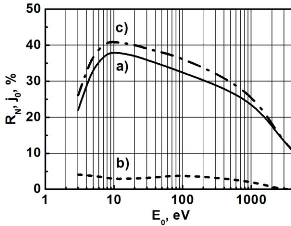
Fig. 2. a) The reflection coefficient  $R_N$ ; b) the re-emission coefficient  $j_0$ ; c) the total coefficient  $R_N + j_0$  are the functions of kinetic energy  $E_0$  of H atoms impinging on the stainless steel surface
