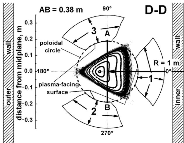
Fig. 1. The poloidal cross-section D-D.  $R$  is a major radius of the torsatron. The magnetic flux surfaces are located between the casings 1, 2, and 3. The vertical diameter  $AB$  of a poloidal circle connects the casings 2 and 3
