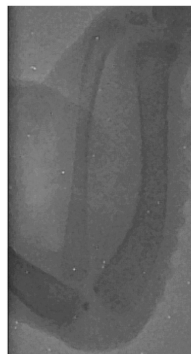
Fig. 8. X-ray image of the biological test object (chicken wing) obtained by using the scintillation panel based on ZnSe with dispersion of the scintillation particles of 80–100 \mu\text{m} .
