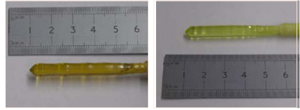
Fig. 2. (Color online) As grown boules of \text{SrHo}_2\text{O}_4 (left panel) and \text{SrDy}_2\text{O}_4 (right panel) single crystals, using growth speeds of 6 to 8 mm/h. Figure is from Ref. 10.
