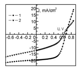
**Fig. 5.** *I-V* characteristic CdTe solar cell with 1- $\mu$ m thick absorber: (1) front ( $V_{oc} = 676 \text{ mV}$ ,  $J_{sc} = 19.7 \text{ mA/cm}^2$ , FF = 60.5%,  $\eta = 8\%$ ) and (2) back ( $V_{oc} = 622 \text{ mV}$ ,  $J_{sc} = 12.2 \text{ mA/cm}^2$ , FF = 43%,  $\eta = 3.2\%$ ) illuminated ones.
