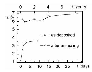
**Fig. 1.** Accelerated lifetime stability tests of an ITO/CdTe/CdS/FTO solar cell (before and after annealing at 350 °C).
