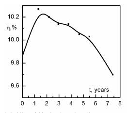
Fig. 4. Stability of thin absorber solar cells.
