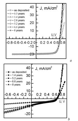
**Fig. 3.** *I-V* characteristic front-illuminated (a) and back-illuminated (b) 2.7 - µm CdTe.
