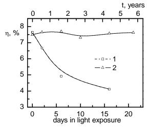
**Fig. 2.** Accelerated lifetime stability test of ITO/Cu/CdTe/CdS/FTO solar cells with 3 nm copper deposition (1) and less than 0.5 nm copper deposition (2).
