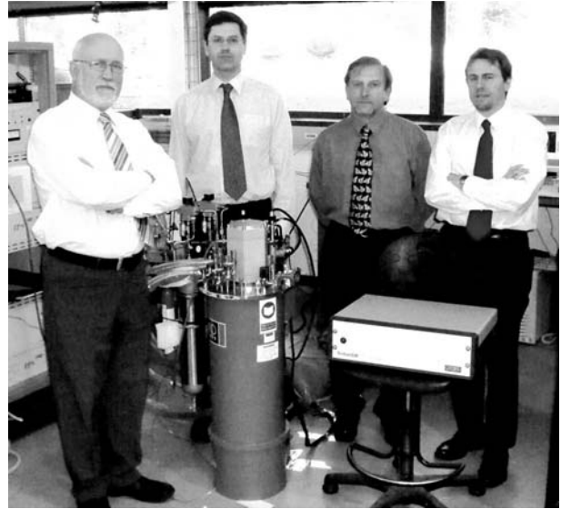
Fig. 6. TritonDR and electronic control box. The core team members are shown to give an idea of the scale of the system.
