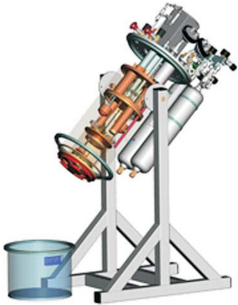
Fig. 2. Transparent view of TritonDR, showing a conceptual design of the support structure, enabling the cryostat to be tilted and positioned for easy access to the sample platform on the mixing chamber.
