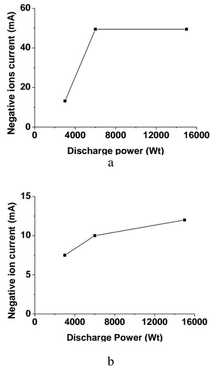
Fig. 5 Dependencies of total negative ion current with  $14^\circ$  propagation angle at 8 cm distance from the source aperture (a) and hydrogen negative ion current with  $12^\circ$  propagation angle at 50 cm distance from the source (b) on power introduced into the discharge
