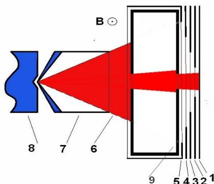
Fig. 2. Scheme of hydrogen negative ion beam current measurement at 8 cm distance from the source aperture: 1-5) collectors for measurements of the beam current components; 6) hydrogen negative ion beam; 7) extracting electrode of the source; 8) anode of the source; 9) additional electrode with two parallel slits
