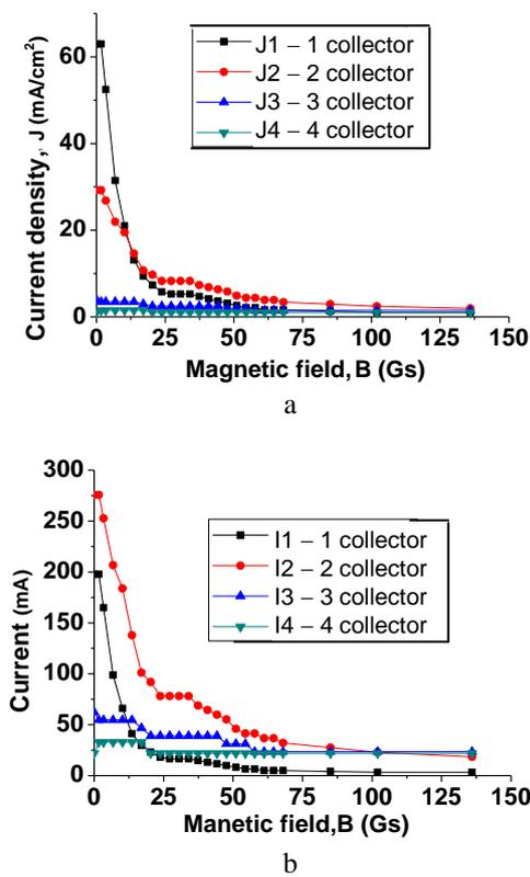
Fig. 4. Dependence of current density onto collectors on magnetic field strength. The discharge current is 30 A (a); Plot of averaged total current onto lamella obtained by multiplying the current density by each lamella area (b)
