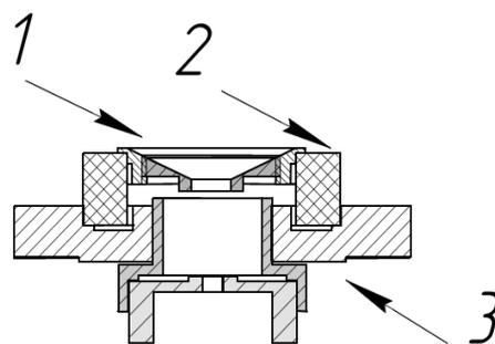
*Fig. 1. Scheme of the ion optics system of the source:
