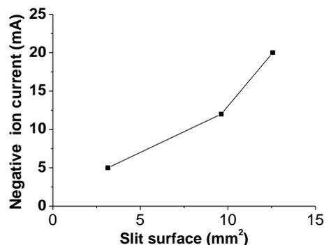
Fig. 7. Dependence of current onto remote collector from the source with anode holes of 2, 3.5, and 4 mm diameter on output slit surface. Pulsed discharge power is 15 kW
