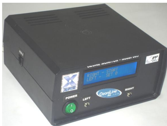
Fig. 1. OCM-003 ozone concentration meter
