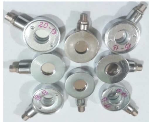
Fig. 2. General view of the surface-barrier detectors manufactured on the basis of Si plates: a – \rho = 1.5 \dots 2 \text{ k}\Omega\text{-cm} , W = 200 \mu\text{m} ; b – \rho = 4 \text{ k}\Omega\text{-cm} , W = 100 \mu\text{m}
