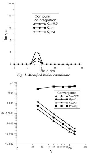
Fig. 2. The relative error in electric fields at the area where the integration contour is at real axis compared with the calculation without analytical continuation. The curve 'penalty' corresponds to applying the penalty method in the area
