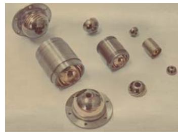
Fig. 2. Elements of the gas dynamic bearing with DLC coatings (convex hemispheres) and with TiN coatings (concave hemispheres)
