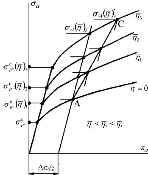
Fig. 6. Cyclic stress–strain diagrams for metals taking into account the stress gradient effect.
