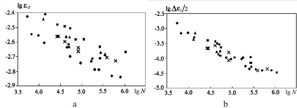
Fig. 5.  $\lg \varepsilon_a$  vs  $\lg N$  (a) and  $\lg \Delta \varepsilon_i/2$  vs  $\lg N$  (b) relations for steel 30KhGSA: ( $\blacklozenge$ ) smooth specimens, ( $\blacksquare$ ,  $\blacktriangle$ ,  $\times$ ) specimens with theoretical stress concentration factors  $K_t = K_t = 2.27, 2.06$ , and  $1.23$ .
