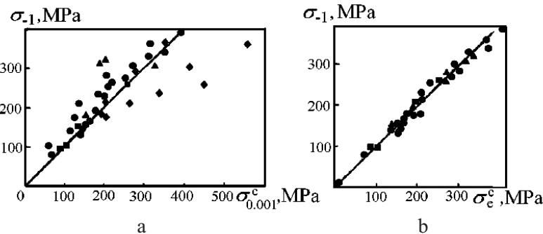
Fig. 2. Comparison of the fatigue limits and cyclic elasticity limits of materials of different classes with common (a) and differentiated (b) offset strain values: (●) carbon and alloy steels; (▲) austenitic steel; (◆) copper-based alloys.
