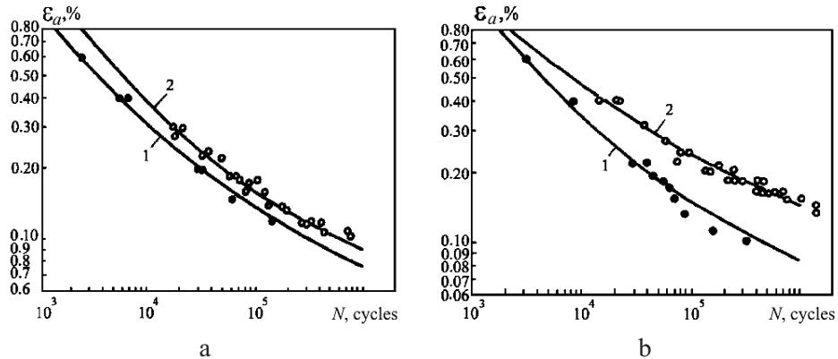
Fig. 4.  $\varepsilon_a$  vs  $N$  relations under symmetrical tension for coarse-grained (a) and fine-grained (b) steels: (1) smooth specimens, (2) specimens with stress concentrators  $K_t = 1.54$  and  $2.57$ .
