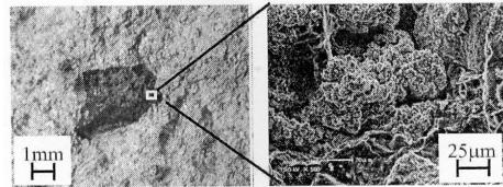
Fig. 1. Oxide inclusion appeared on fracture surface [1].
