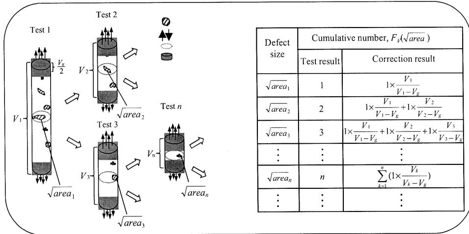
Fig. 4. Correction method.
