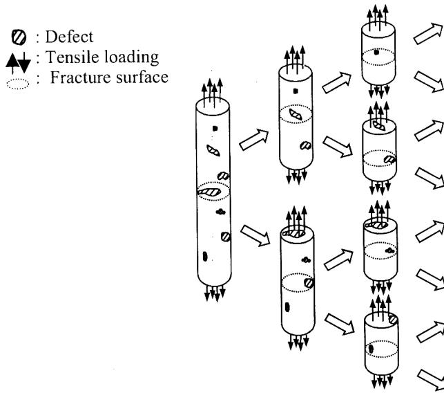
Fig. 2. Schematic diagram of the repetitive tensile test.
