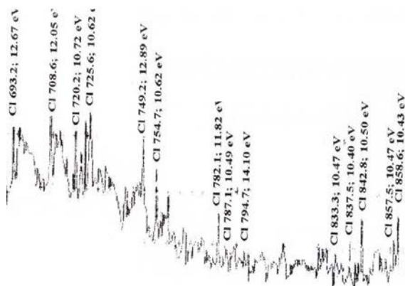
Fig. 8. The emission spectrum of the plasma at U_{bias} = -120 V
