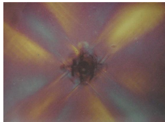
Fig. 3. The picture of residual stress distribution around the seat of a local heat burst and the formed pore; obtained by the method of photo-elasticity in circulairement polarized light
