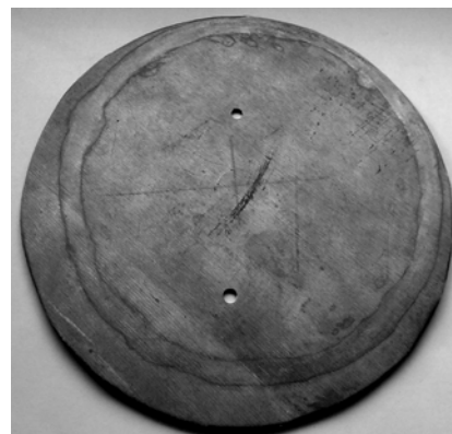
Fig. 4. Ring beam track on a copper target with diameter 140 mm at the microsecond output
