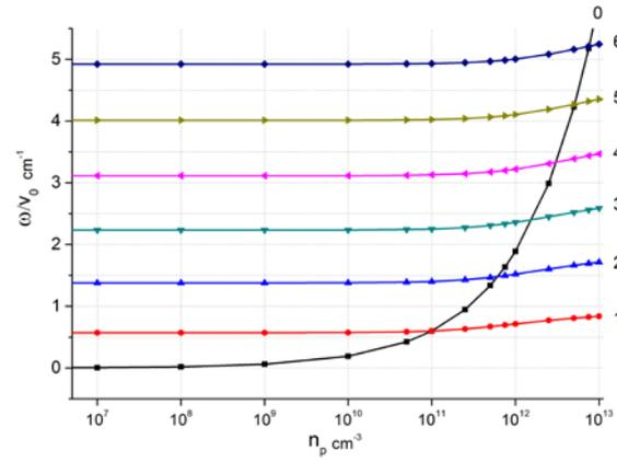
Fig. 2. Eigen frequencies of plasma-dielectric structure depending on plasma density: curve 0 – plasma wakefield; 1-6 – the first 6 solutions of dispersion equation (8) and (12) for  $\omega_s$
