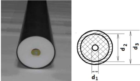
Fig. 18. Dielectric waveguide of circular cross-section;  $d_1=21.1$  mm;  $d_2=85$  mm;  $d_3=89$  mm
