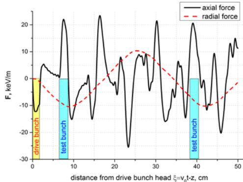
Fig. 3. Axial profile of longitudinal (solid line) and transverse (dashed line) forces, acting on accelerated bunch located at a distance 0.95 cm from the structure axis
