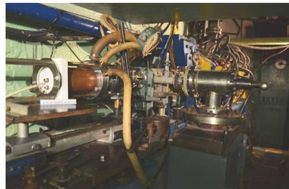
Fig. 21. Scheme of experimental setup: 1 – accelerator “Almaz-2M”; 2 – titanium foil; 3 – leak valve; 4 – dielectric waveguide; 5 – matching dielectric cone; 6 – ferrite absorber; 7 – microwave probe; 8 – oscilloscope GD-840S; 9 – double Faraday cup; 10 – vacuum pump
