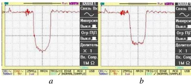
Fig. 14. Oscillograms of electron beam current on accelerator exit: focusing lens switched on (a); focusing lens switched off (b)
