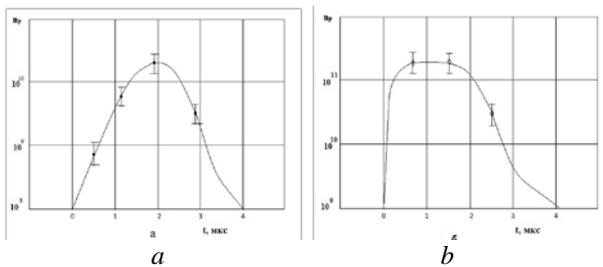
Fig. 22. Temporal dependence of the plasma density formed by injecting bunches through the neutral gas at pressure of  $P = 600$  Torr: without (a), and with dielectric (b)
