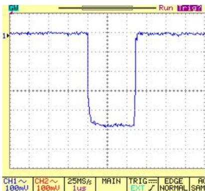
Fig. 9. Oscillogram of the envelope of the microwave signal of the master-oscillator
