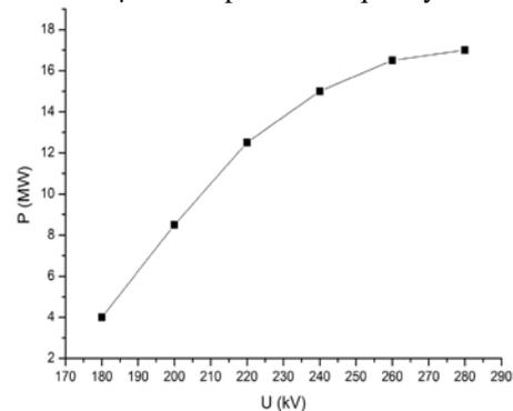
Fig. 10. The the output pulse power of the klystron dependence of upon anode voltage
