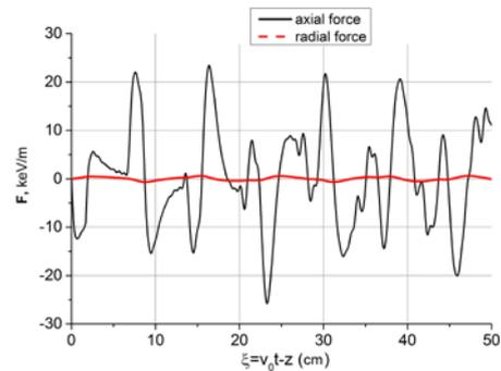
Fig. 5. Axial profile of longitudinal (black line) and transverse (red line) forces of dielectric wakefield, acting on accelerated bunch located at a distance 0.95 cm from the structure axis
