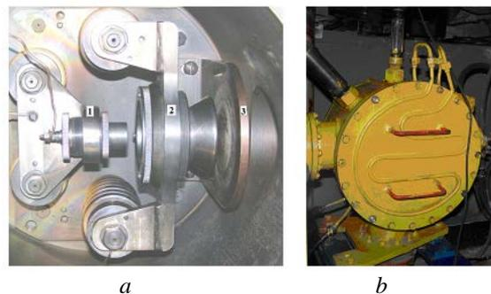
Fig. 7. Electron gun: 1 – unit of electron beam heater of the cathode; 2 – cathode unit; 3 – anode (a); b – electron gun chamber (b)
