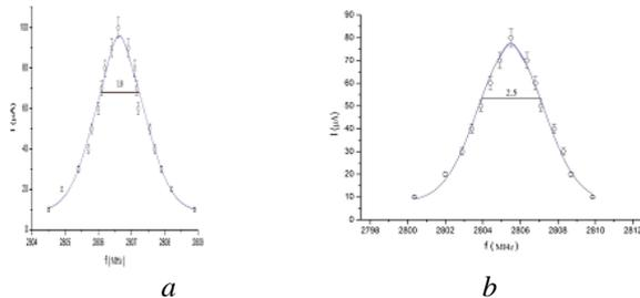
Fig. 19. Resonance curves for: resonator without (a), and with insert (b)
