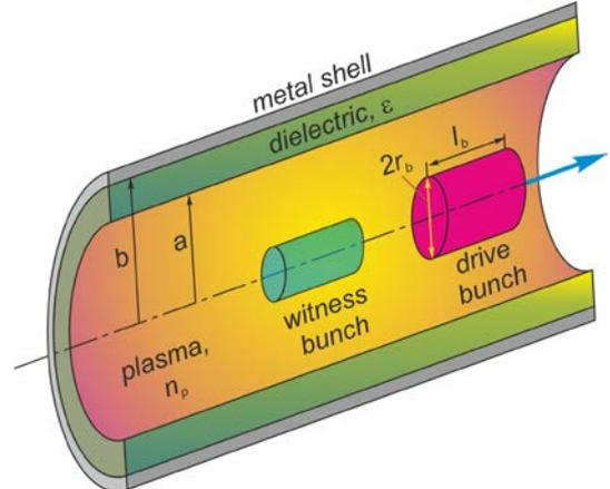
Fig. 1. Geometry of plasma-dielectric wakefield accelerating structure
