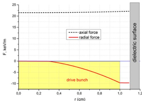
Fig. 4. Transverse profile of longitudinal (solid line) and transverse (dashed line) forces, acting on the accelerated bunch, located in the first maximum of accelerating field at a distance 7.562 cm from the head of driver-bunch
