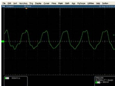
Fig. 20. Oscillogram of wakefield excited in a dielectric waveguide
