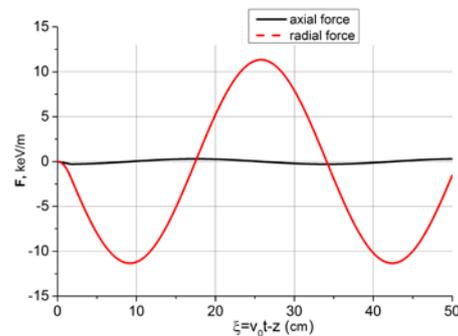
Fig. 6. Axial profile of longitudinal (black line) and transverse (red line) forces of plasma wakefield, acting on accelerated bunch located at a distance 0.95 cm from the structure axis
