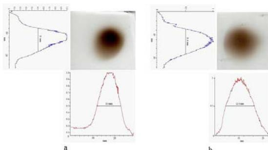
Fig. 15. Beam imprints on the glass plates located at the accelerator exit in vertical (left) and horizontal (below) planes: focusing lens switched on (a); focusing lens switched off (b)
