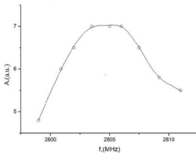
Fig. 8. Dependence of amplitude of the microwave signal upon master-oscillator frequency
