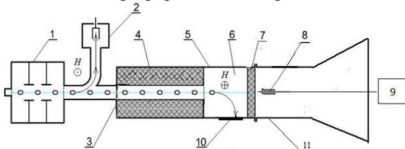
Fig. 13. 1 – accelerator "Almaz-2M"; 2 – magnetic analyzer; 3 – diaphragm; 4 – dielectric structure; 5 – waveguide; 6 – traversal magnetic field; 7 – vacuum teflon plug; 8 – microwave probe; 9 – oscilloscope; 10 – metal collector; 11 – waveguide with a horn
