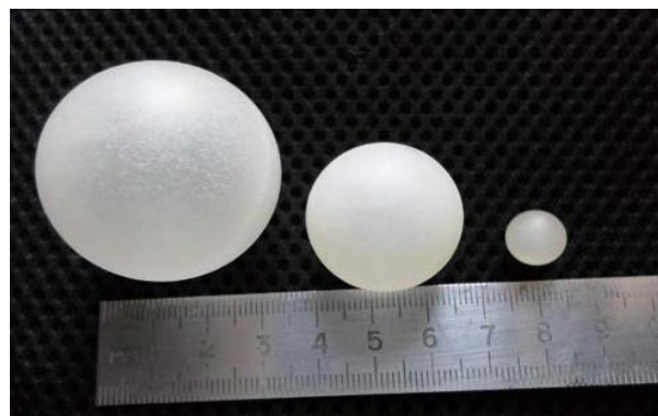
Fig. 4. Balls from a composite material for protective layer filling
