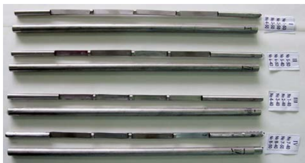
Fig. 6. The view of the consoles with the samples and the pipes of the four-channel irradiation cell
