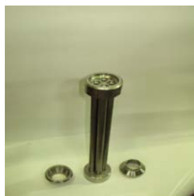
Fig. 5. The view of the four-channel irradiation cell. The material cell is stainless steel 12X18H10, the thickness of the cell wall – 2 mm, external pipe diameter – 14 mm
