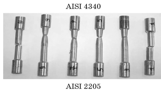
Fig. 7. Macrophoto of tensile test results of friction-welded joints.
