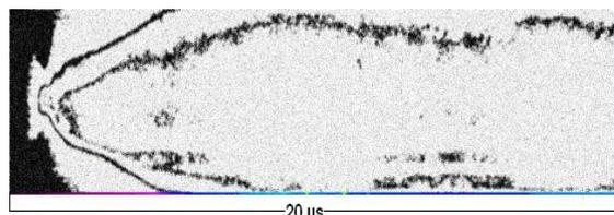
Fig. 3. Time scanning of discharge luminescence for long pulse mode
