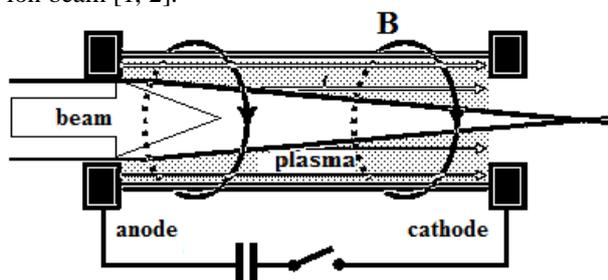
Fig. 1. Ion focusing in a plasma lens
