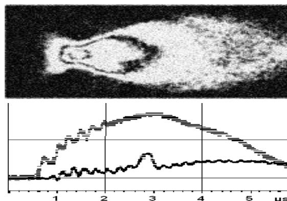
Fig. 2. Time scanning of discharge luminescence and discharge and beam currents for short pulse mode
