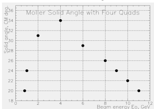
Fig. 4. Acceptance of polarimeter by solid angle \theta_{cm} for configuration with four quadrupole magnets
