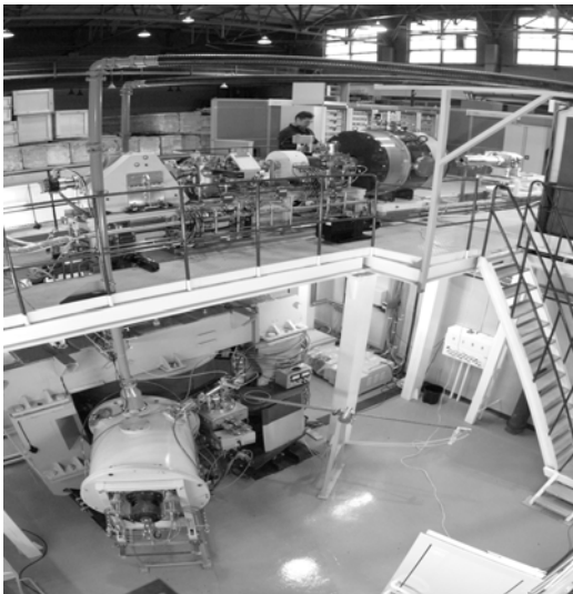
Fig.1. IC100 cyclotron. Shown are the SC ECR source, injection line, magnet and resonance cavity
