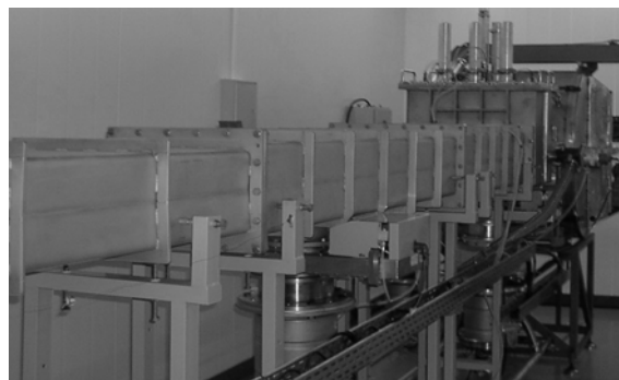
Fig.8. Beam delivery line to device for polymer films production
