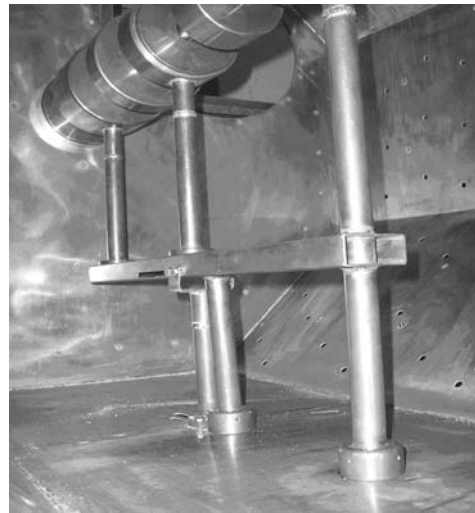
Fig.4. The end resonant tuning element on the exit end accelerating structure
