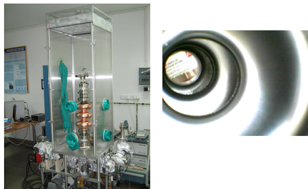
Fig. 11. UHV linear-arc facility and end-on view of a test 3-cell cavity coated with Nb
