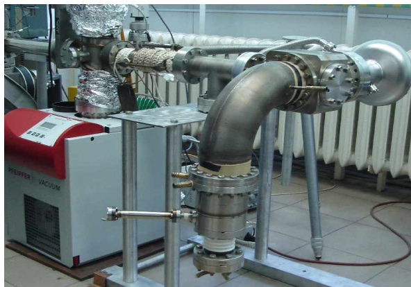
Fig.2. Picture of the planar arc facility equipped with the magnetic filter (without external coils) and the RF Gun
